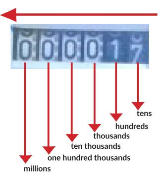
Read the displayed numbers from left to right. Be sure to include the stationary zero. This is your meter reading.
